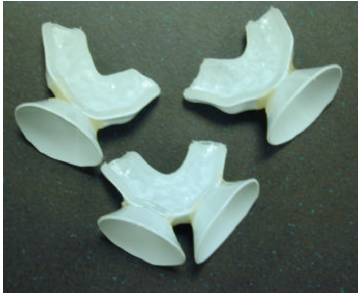
Figure 7. Jigs used to reproducibly place the chromameter head on the buccal surface of the maxillary right lateral, the maxillary left lateral and the maxillary central incisors.
